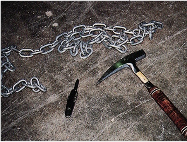
Figure 1. Various tools can be used to evaluate the soundness of a concrete surface. Dragging a chain or tapping a hammer on the surface produces hollow sounds over delaminated concrete. To check for laitance, scrape the surface with a knife.
