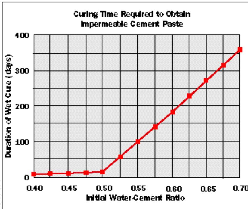
Figure 2. Concrete mixes with water-cement ratios of greater than 0.50 require longer wet-curing times to obtain a relatively impermeable paste. To avoid moisture problems in slabs on grade, try to use low water-cement ratio mixes and provide adequate curing.
