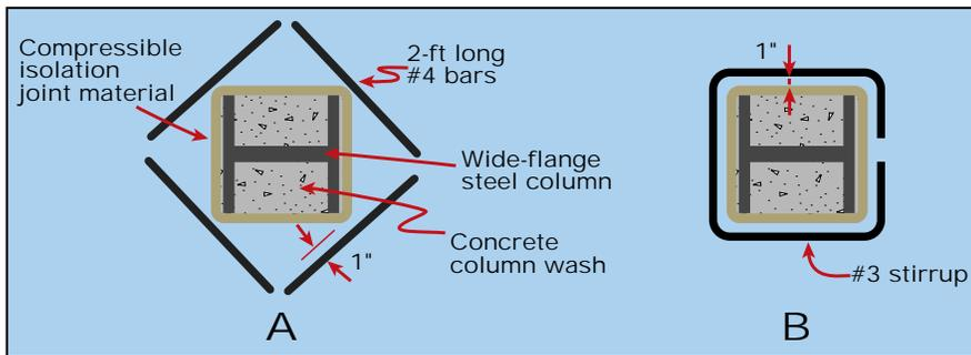
Eliminate the normal isolation-joint box outs at wide-flange steel columns by wrapping the column with compressible material and using 2-foot lengths of #4 bars (A) to control cracking at the reentrant corners. To speed up steel placement at the columns, have the rebar supplier fabricate continuous #3 stirrups that workers can easily bend open to fit around the column (B). In either case, the steel should be positioned with a top-and-side clear cover of 1 inch.
