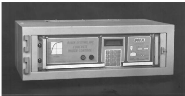
As the aggregate hits the meter, the moisture content is measured and digitally displayed.
