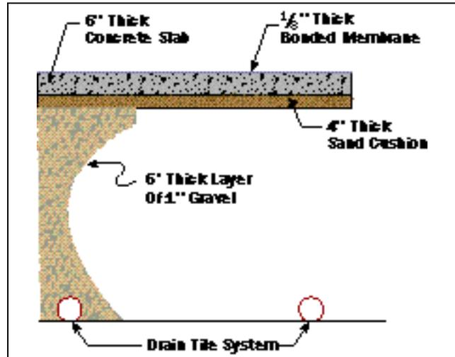
Figure 4. Swimming pool floor construction details.
